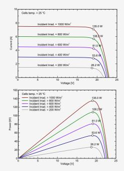
STC: Irradiance 1000W/m<sup>2</sup>,Module temperature 25°C,AM1.5 spectrum.
