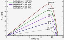
STC: Irradiance 1000W/m<sup>2</sup>,Module temperature 25°C,AM1.5 spectrum.
