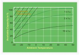
Extracted capacity in relation to the temperature.
