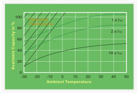
Extracted capacity in relation to the temperature.
